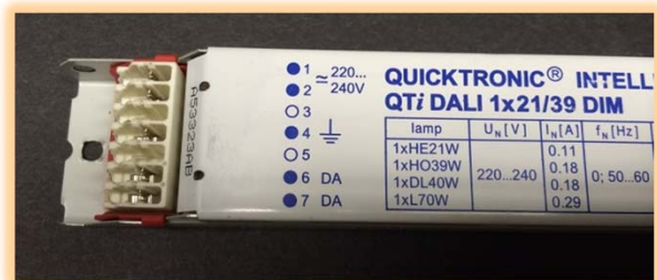
Image 4: Close-up. OSRAM Ballast with DALI Interface
