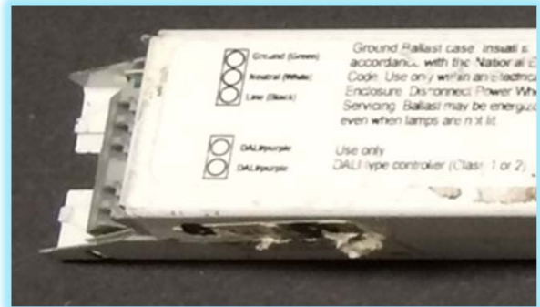
Image 2: Close-up. Sylvania Ballast with DALI Interface
