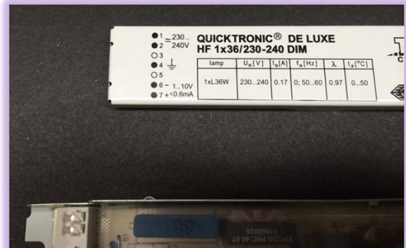
Image 2: Close-up. OSRAM Ballast with 1-10V Interface
