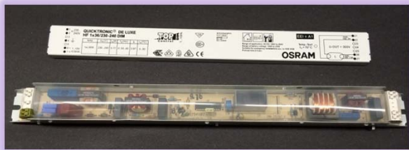
Image 1: OSRAM Ballast with 1-10V Interface
