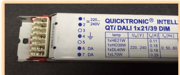
Image 4: Close-up. OSRAM Ballast with DALI Interface
