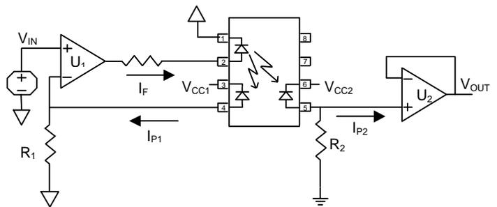
Figure 1: SLC800 in Photoconductive Operation
